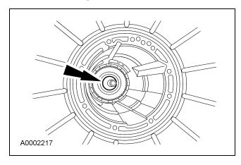
25. Install low/reverse planetary carrier needle bearing (No. 9) onto the output shaft ring gear and hub assembly.
